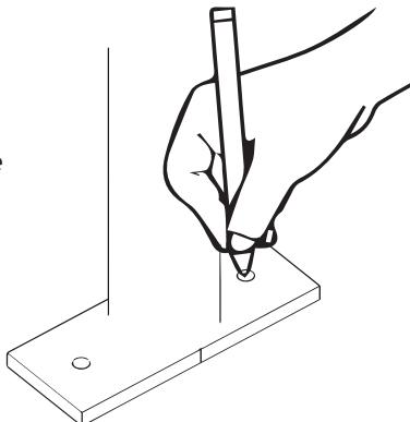
5. Remove nut and washer from anchor and insert all anchors 1 1/2" into drilled holes. Pound all four anchors into surface lightly with mallet or hammer to ensure they will stay in place.
