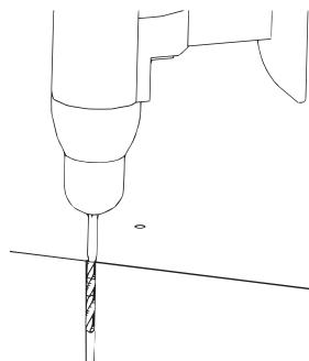
4. Remove the product if used as a template from holes drilled and clean out areas in holes with a vacuum, pipe cleaner or small brush and then clear dust or debris from surrounding area.
